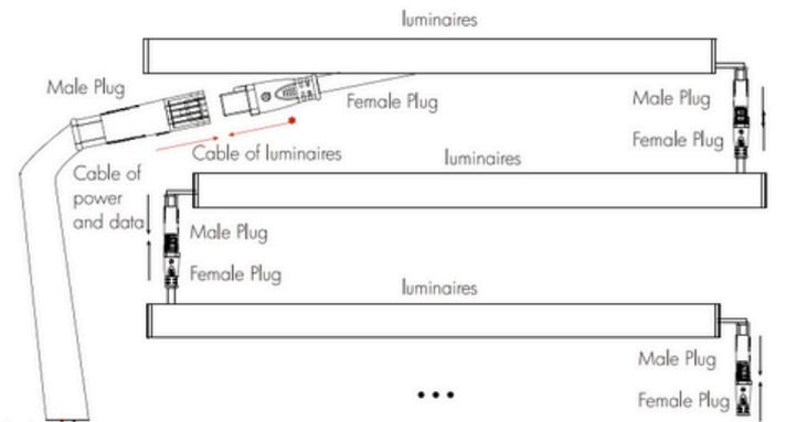
Notice: Use the female plug with end cap, to seal the male terminal of the last luminaires.
