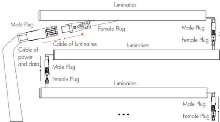
Notice: Use the female plug with end cap, to seal the male terminal of the last luminaires.
