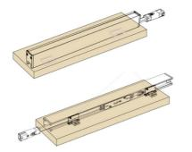
• Adjust, lock the fixation screw and complete
