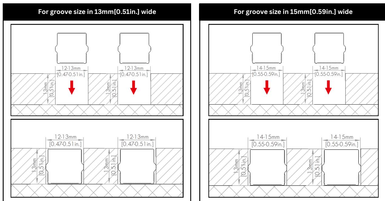
Recessed press-fit installation into the slat groove with no clips, tools, or additional hardware required.
